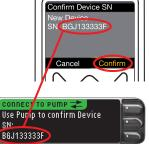
When the pump links to the meter, the SN on the meter screen will change to a different serial number. This number is the **pump** SN.
